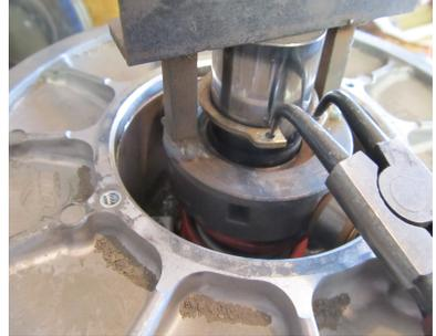
13) \* **Install new helix using selected ramp profile** - Install the proper ramp for your application.
